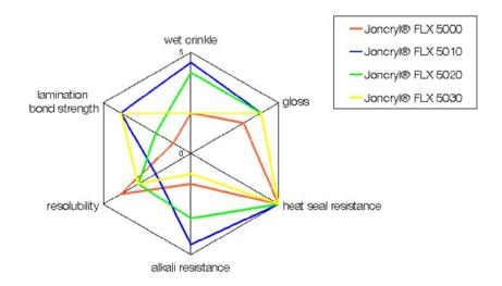
Joncryl® FLX 5030 is developed for water-based lamination inks. A white ink based on Joncryl® FLX 5030 shows a very good leveling and lay. Reverse printed on OPP and laminated with an adhesive it results in laminate structure suitable for the medium-duty laminate segment like bakery, confectionery and snack foods packaging.
